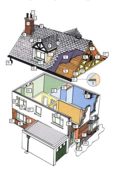
Chimney pots Coping stone 3 Chimney head 4 Flashing Ridge ventilation 5 6 Ridge board Slates/tiles 8 Valley guttering 9 Dormer projection 10 Dormer flashing
